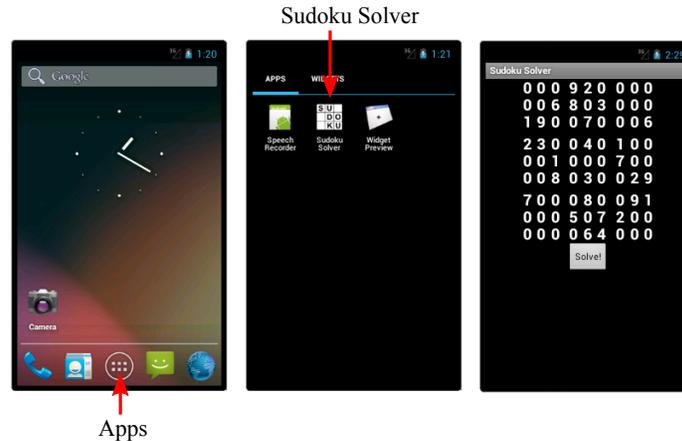
Figure 3: The android emulator. To unlock the emulator click on the lock symbol and drag to the unlocked symbol. To open the Sudoku solver app, select the app menu as shown above, scroll to the right, and double click. In the next part of the lab, we'll add the solve button shown in the final image above.
